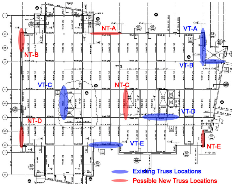
Figure 33 – Existing and New Truss Locations
